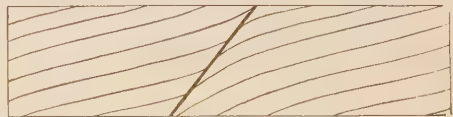
FIG. 268. — Diagram showing "drag dip" near a fault. (Modified after W. N. Rice.)
